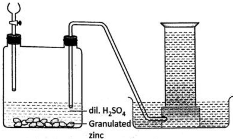
(i) The apparatus is set up for the preparation of a certain gas in the laboratory. Which gas is this?
